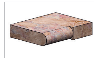
PARTIAL WORK ON BULL-NOSE PROFILE 棋子边分段加工
