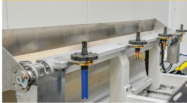
FOUR POSITION MAGNETIC TOOL CHANGER FOR AUTO CHANGING CORE BITS AND ROUTER TOOLS 4位磁力刀具库，用于自动更换钻头或铣刀工具
