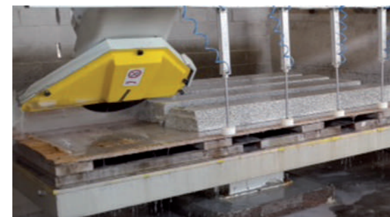
Inclined cuts 倾斜切
