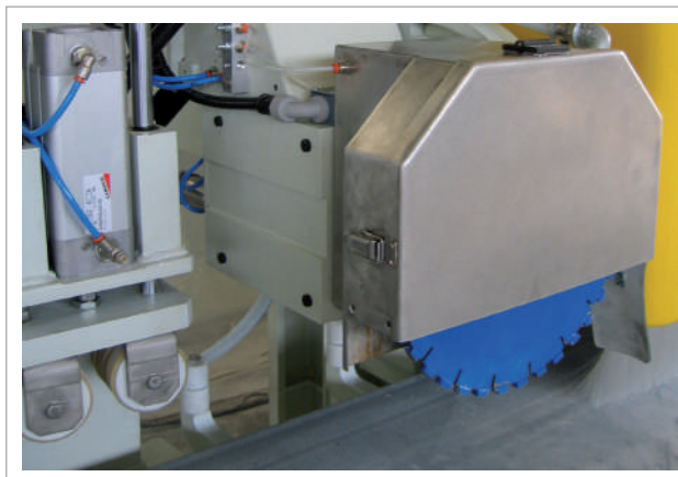
Drip cut unit Gocciolatoio
