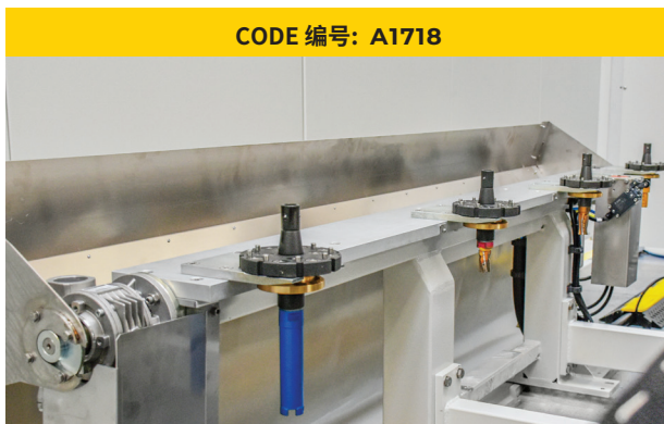
FOUR POSITION MAGNETIC TOOL CHANGER FOR AUTO CHANGING CORE BITS AND ROUTER TOOLS 4位磁力刀具库，用于自动更换钻头或铣刀工具
