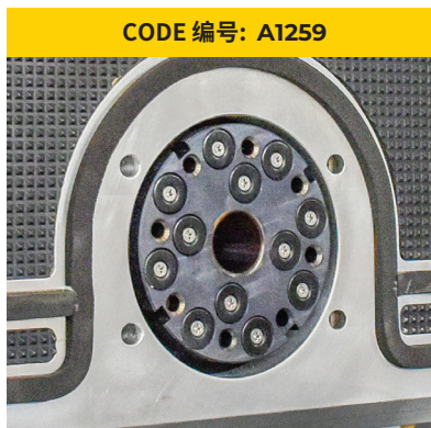
VACUUM BLADE GUARD WITH COOLING TOOL NOZZELS 带冷却工具喷嘴的真空锯片防护罩
